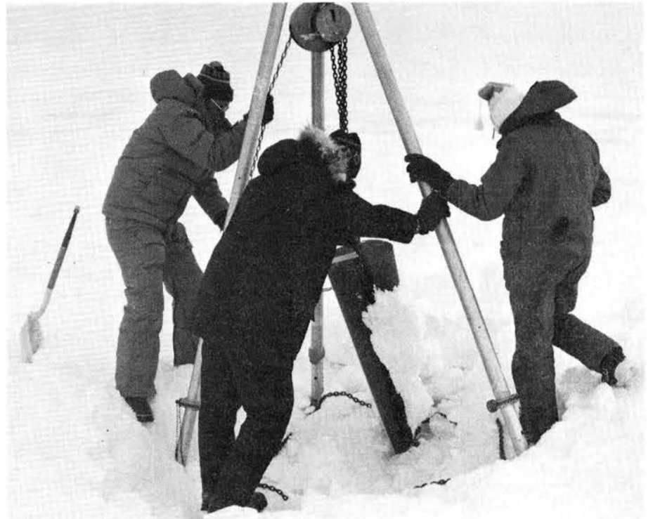
SANDIA EXPERIMENTERS RECOVER an ice penetrator after a drop north of Prudhoe Bay, Alaska. The penetrator bores through several tens of feet of ice when dropped from a few thousand feet altitude.
